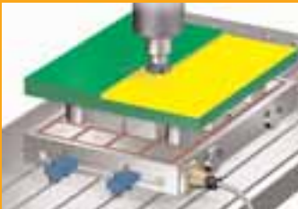
• rough-milling the 1st surface
