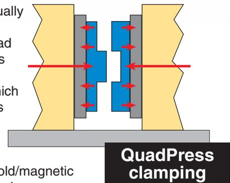
The combination of mold/magnetic module/machine platen becomes a perfect match and guarantees superior operating conditions. The absence of deflections in the mold and machine platens translates to better quality and repeatability of the molded parts.
