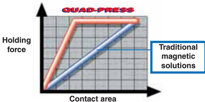
The innovative polar geometry of QuadPress can reach the maximum operating efficiency even on molds of smaller size being the polar area concentrated in the inner surface of the magnetic module corresponding almost to the size of the smallest mold acceptable by the machine.
